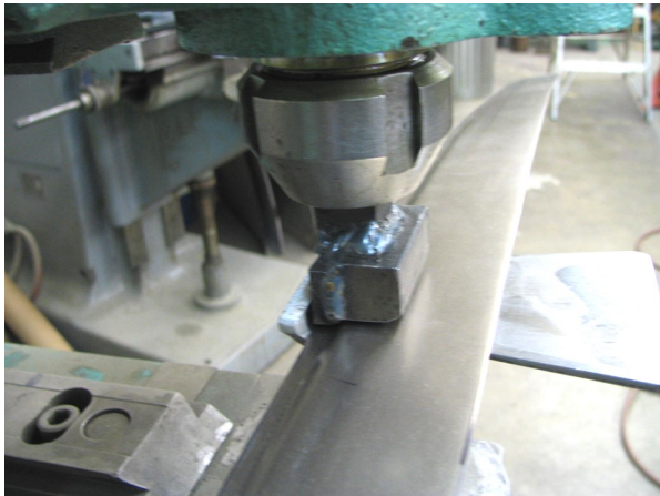
Fig. 9.11. Making an offset on 2" wide strip of metal
